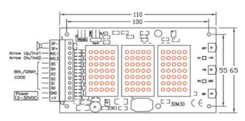
3DM30 is a microcontroller based dot matrix display device for lifts. It can be assembled either to the car or to the level. It can present floor markings, direction arrows and indicators. It accepts wide range of nominal supply voltages, because it is equipped with high efficiency switched mode power supply. 3-tone gong sound generator produces different sound depending on direction. Advanced digital filtering enhances robustness in poor signal quality environments.
